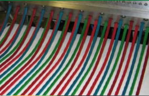
Extrufood excels in the manufacturing of dies for the confectionery industry. Well known are the dies for belts, spaghetti strands, ropes and cables for single or multi-colored extruded products which can be either solid, hollow or filled.
