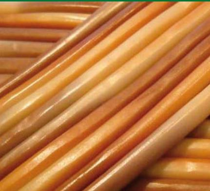
Not only 6 different colors simultaneously in strands next to each other, but also switching colors within each strand during the extrusion is possible. This will give the industry a new boost, as new combinations can be made, more products can be made on one line, so greater flexibility and a higher efficiency are achieved!
