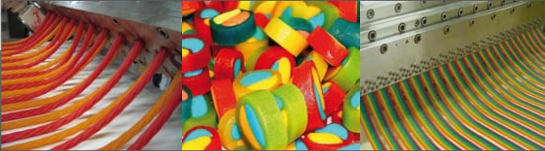
Extrufood was the first to offer multi-color confectionery production lines with the introduction of the Diemix<sup>®</sup>. The Diemix<sup>®</sup> enables the production of licorice or fruit gum with up to 6 different colors simultaneously while using only one extruder.
