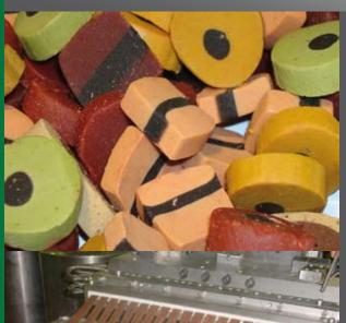
The rotary dies and fixed dies enable the production of pet snacks & treats with almost endless possibilities for combinations of colors, shapes and textures, twisted or non-twisted, co-extruded or hollow.
