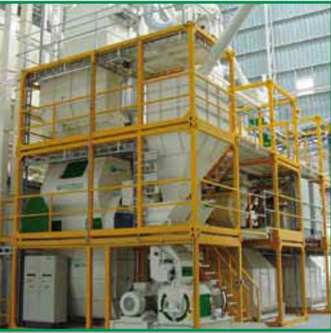
At Wynveen International we can install your choice of pelletizer or extruder in your installation. We match the dosing screws and conditioners to the circumstances on site to ensure optimum dosing and conditioning prior to further processing in the pelletizer or extruder.
