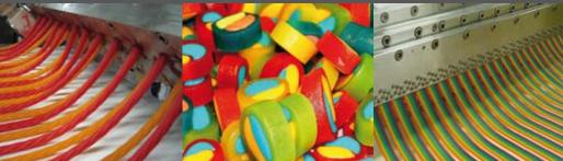
Extrufood was the first to offer multi-color confectionery production lines with the introduction of the Diemix<sup>®</sup>. The Diemix<sup>®</sup> enables the production of licorice or fruit gum with up to 6 different colors simultaneously while using only one extruder.
