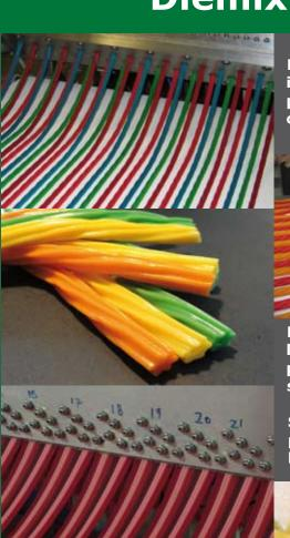
Extrufood excels in the manufacturing of dies for the confectionery industry. Well known are the dies for belts, spaghetti strands, ropes and cables for single or multi-colored extruded products which can be either solid, hollow or filled.
