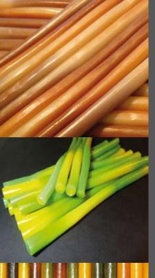
Not only 6 different colors simultaneously in strands next to each other, but also switching colors within each strand during the extrusion is possible. This will give the industry a new boost, as new combinations can be made, more products can be made on one line, so greater flexibility and a higher efficiency are achieved!
