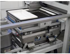
The ALFRA FCD Flexible Component Dosing System uses a dosing plateau with ALFRA Dosing Slides. Therefore it very accurately doses large and small quantities.
