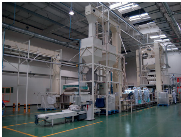
Simatek Universal Elevators conveying sunflower seeds in China. Photo: Sunshine Produce Ltd., China
